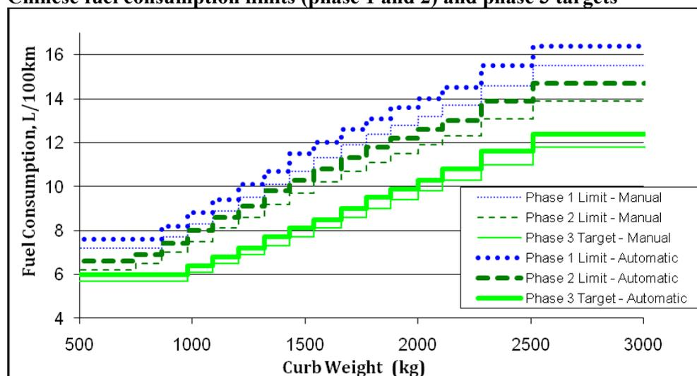
45. As mentioned, the Chinese standard is a weight-based standard that every domestically made vehicle in China must achieve. Vehicles that do not meet the standard are not permitted to be sold. The testing protocol is based on the European NEDC testing standard system, using a test vehicle to measure carbon dioxide emissions over a test cycle, then converting the value into fuel consumption in L/100 km.
